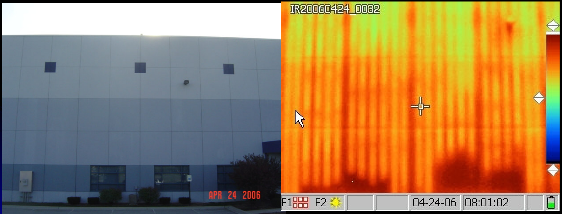
Photo shows distinct lines of the cables in the precast masonry wall
